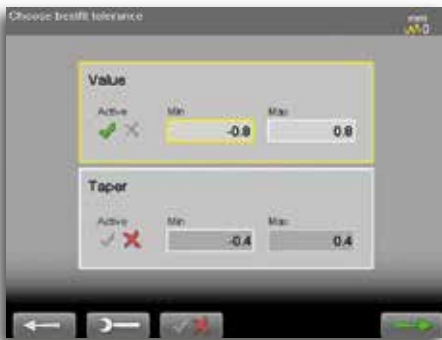
Set tolerance values for flatness and taper.
