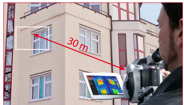
Determining the appropriate distance to the measuring object based on the measurement spot size
