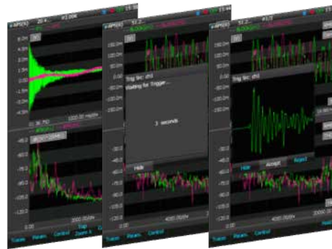
Figure 5: Acquisition Modes 'Free-Run', 'Auto-Trigger', and 'Manual Trigger'
